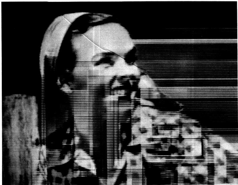
Fig. 1—Effect of 10^{-4} channel bit error probability on output picture: Graham 3 bit/pel codec.
